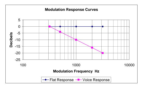
The above plot shows the response in decibels vs. log of modulation frequency for the flat and voice response. These are the modulation response curves used for all the other plots.
