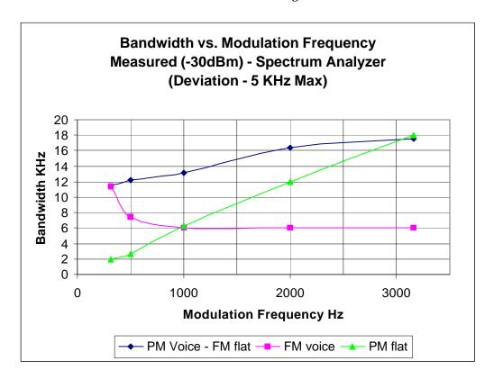
My textbooks did not indicate what the level in dB down from the carrier is for the bandwidth that is calculated using the Carson Rule. My estimation for the bandwidth was – 30 dBm below the carrier, which is what I used for my measurements.
