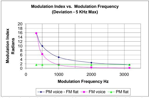
The above plot, of modulation index vs. modulation frequency, was made with the condition that the maximum deviation was 5 KHz. Because the voice amplitude response is a maximum at low frequencies (for this plot, the low frequency is 316 Hz), the modulation index is lower as modulation frequency increases. Note that the overall modulation index for PM voice is higher than FM voice and thus the PM modulator better utilizes the voice response for higher modulation efficiency.
