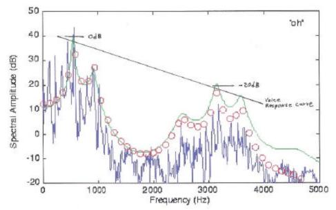
The above plot of the voice response for the word "oh" is very typical of what a human voice spectrum components look like. Thus for the FM communication systems, the modulation input is a voice response that has a 6 dB per octave or 20 dB per decade sloping response. An examination of the audio clipper circuit in a NBFM transmitter will reveal that it operates on the basis that this is the expected input response.
