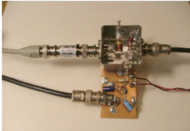
Photo of LC Modulator Test Circuit
